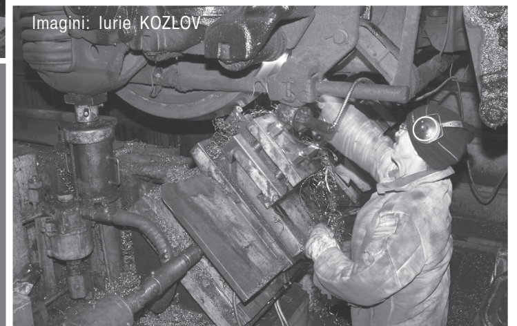
Are loc strunjirea osiilor montate
